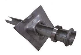
The Friction bolt utility hangers available in all Models and up to 900mm. They're not for ground support, but they offer the same installation advantages as friction bolt Stabilisers. They come in the same tube diameters, and use the same bearing plates. They are used to support cables, ductwork, pipes and Mine Mesh. Lightweight items such as ventilation tubing may be hung from the loop on the bearing plate.
